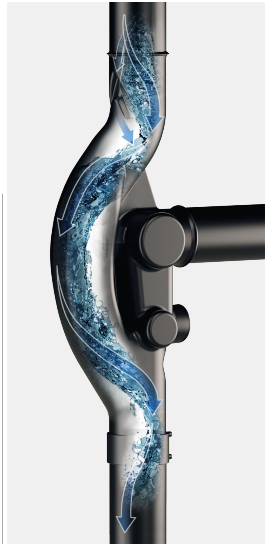
↑ This graphic visualization of the Sovent fitting is based on the data from the computer simulation.
